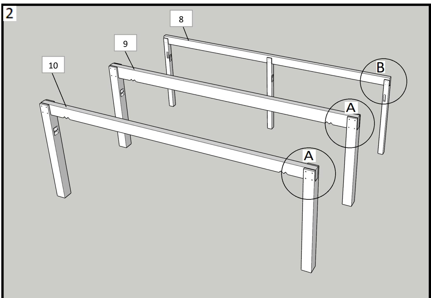
NB! Push the bolts through the pre-drilled holes, add washers and nuts. If there are differences in the holes, drill the holes with a 16-18mm drill. Do not tighten the bolts before the diagonal ties (part 14) are attached according to the instructions! Then tighten the bolts firmly.
